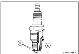
A. Spark Plug Gap B. Electrodes
