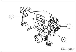
B. Control Lever (Throttle) H. Choke Valve Pivot Arm I. Throttle Valve Pivot Arm
