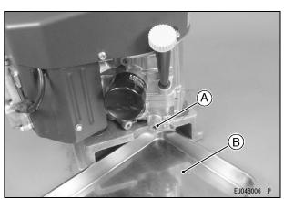
A. Oil Drain Plug B. Suitable Container
