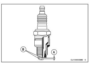
A. Spark Plug Gap B. Electrodes
